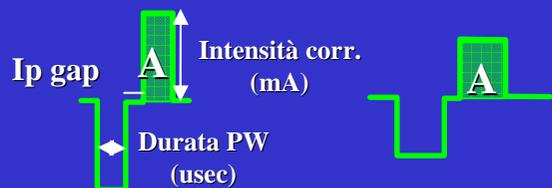
$$\text{Area} = \text{Carica}_{\text{Coulomb}} = \text{Int}_{\text{corr el}} \times \text{Durata}_{\text{PW}}$$
