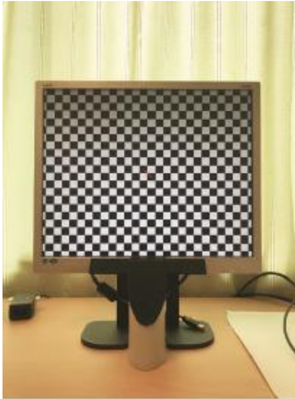
Fig. 2.4 LED backlit LCD graphic stimulator
